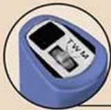
**3** A transmitting coil sends the coded signals as radio waves to the cochlear implant under the skin.
